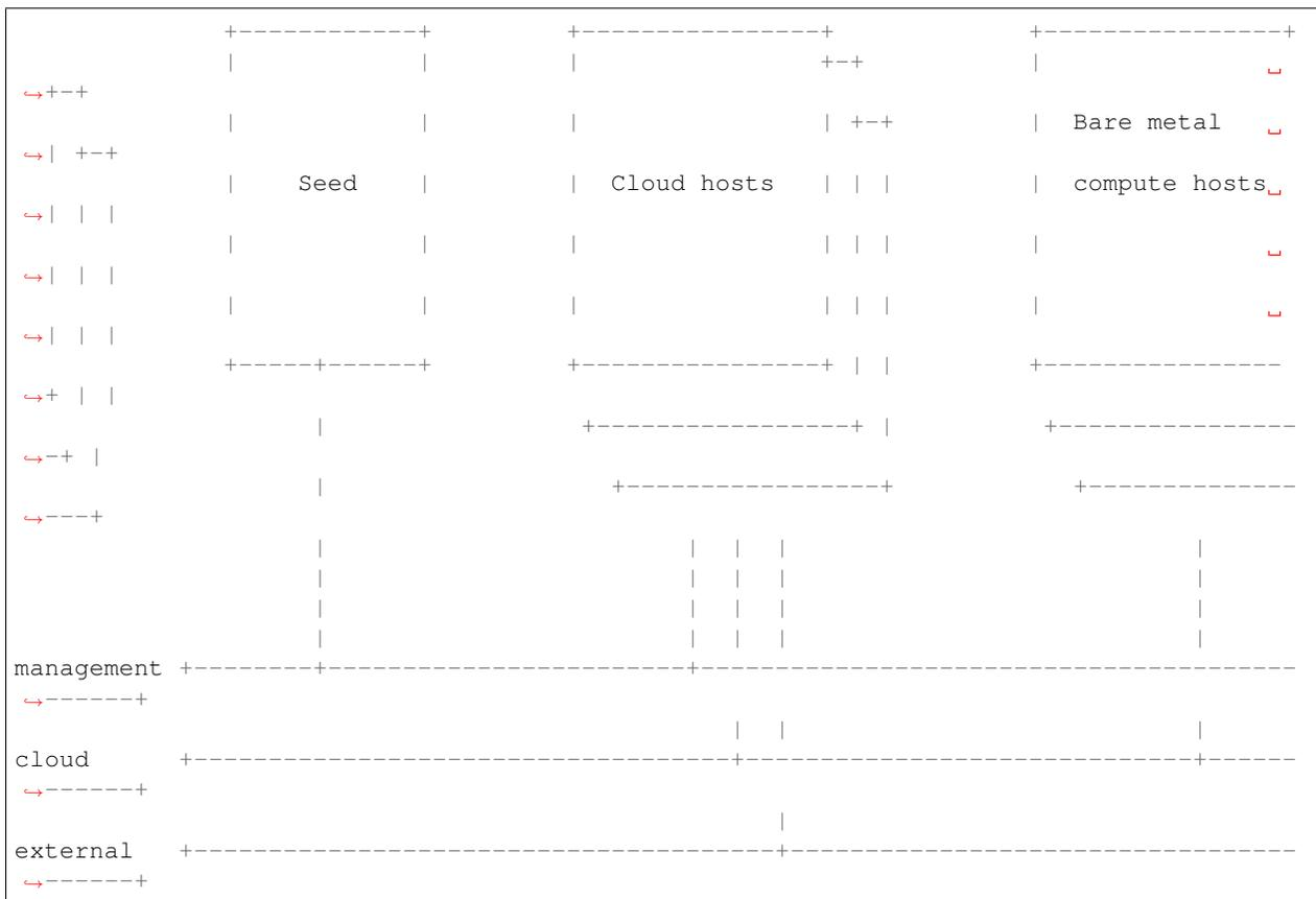
The management network is used to access the servers’ BMCs and by the seed to provision the cloud hosts. The cloud network carries all internal control plane and storage traffic, and is used by the control plane to provision the bare metal compute hosts. Finally, the external network links the cloud to the outside world.
